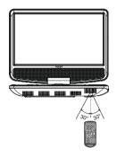
Approximate working distance is 3 metres with a working angle of 30° left and right from centre.
